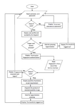
Fig. 3. Flowchart of IOT based smart public distribution system
