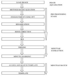
Fig. 4. Steps involved in fingerprint recognition.
