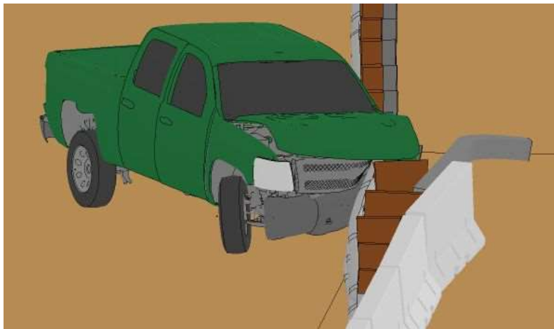
Figure 66. Vehicle Snag on Blockout, Impact Location No. 6 at 90 ms
