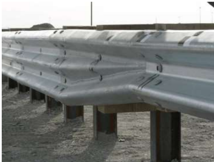
Figure 19. MGS Stiffness Transition with Asymmetrical Element [21]
