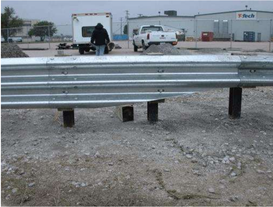
Figure 18. Asymmetric Transition Element for Test No. MWT-4 [21]
