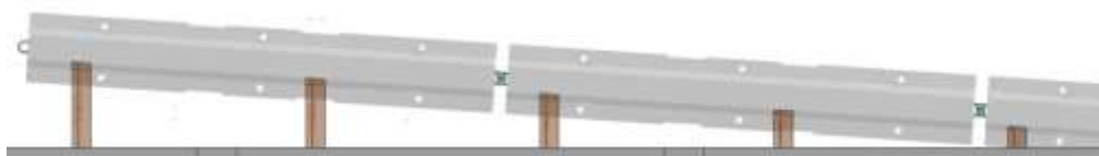
Figure C-4. Blockout Connection to PCBs
