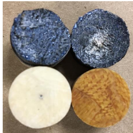
Figure 6. A S/DG-UHTR F2 Sample pre-test (bottom left) post-test (top left) and a MX2600 Sample pre-test (bottom right) post-test (top right)
