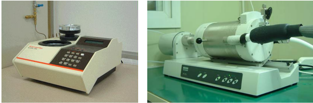
Figure 9. Instruments; (a) pycnometer, (b) dilatometer
