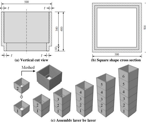
(c) Assembly layer by layer Figure 1. Illustration of the SIP formwork system.
