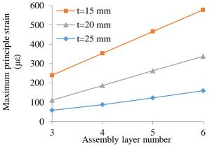
Figure 4. Effects of assembly layer number and wall thickness on maximum principle strain.
