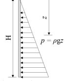
Figure 2. Illustration of static hydraulic pressure applied on SIP formwork.
