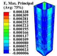
Figure 3. Distribution of maximum principle strain.
