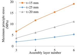
Figure 6. Effects of assembly layer number and wall thickness on maximum principle stress.
