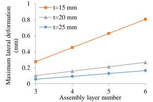
Figure 8. Effects of assembly layer number and wall thickness on lateral deformation.
