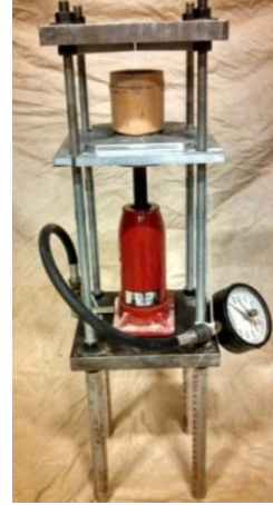
b) set-up for longitudinal shear test
