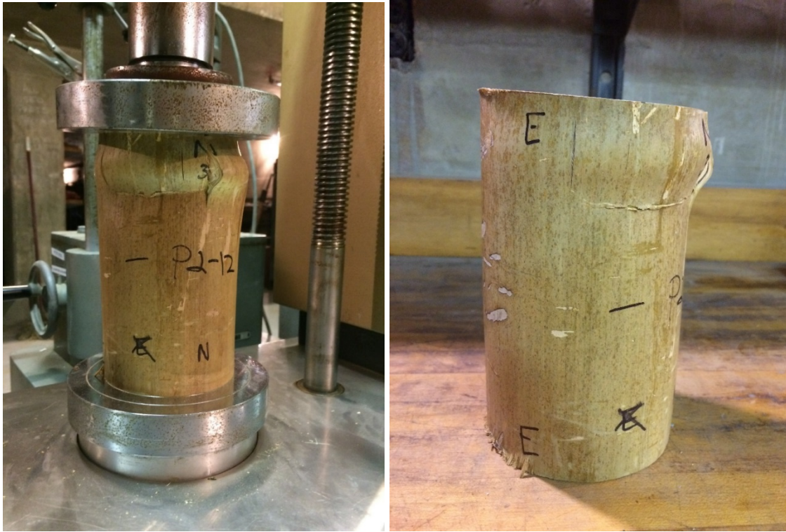
Figure 17: Non-parallel-end compression specimens.
