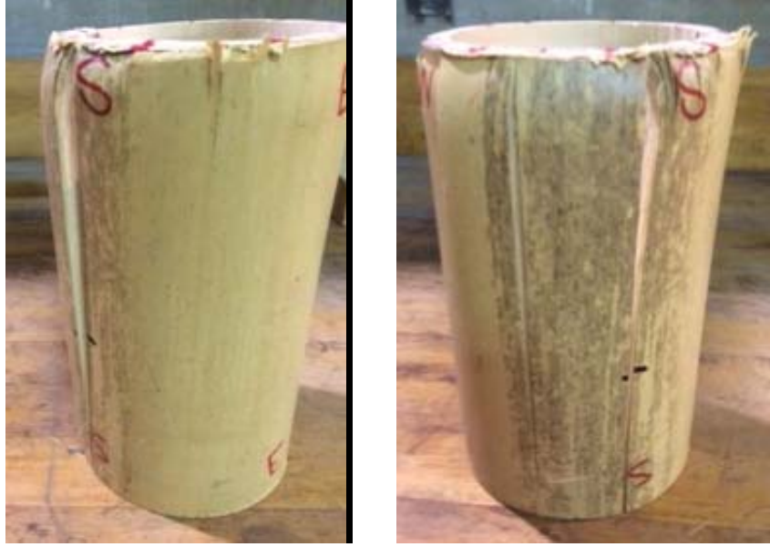
Figure 18: Local crushing evident in out-of-plane specimens.
