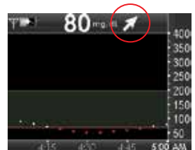
Rate of change arrow appears in upper right of trend graph
