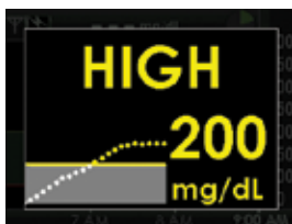
High glucose alert set at 200 mg/dL
