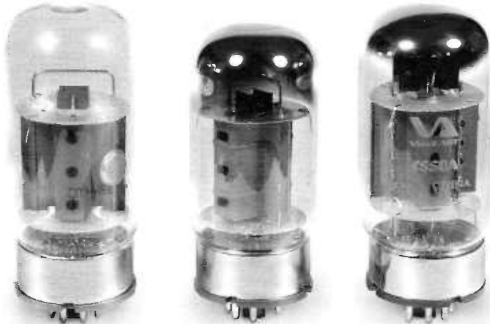
Svetlana SV6550B (early 1990s with pill getter), Svetlana SV6550C (2001) and Valve Arts Chinese 6550CA (2002)
