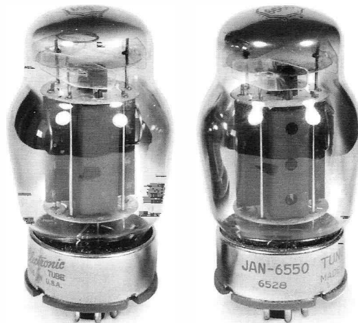
Tung-Sol 6550 (1963 triple getter-no holes with GE markings) and Tung-Sol 6550 (1965 triple getter-with holes)
