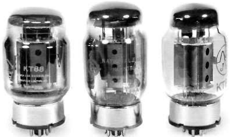
Chinese KT88 (1990s branded Penta Labs), Richardson-made KT88 (1996) and JJ KT88 (2002) (Slovakian-made)
