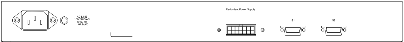
Figure 1-13 Rear panel view of the DGS-3120-24TC
