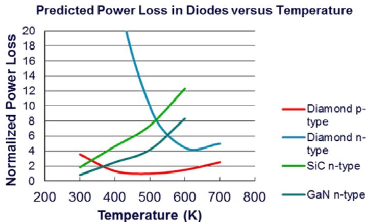
*Comparison of diodes designed to flow the same current and block the same high reverse bias voltage.*
