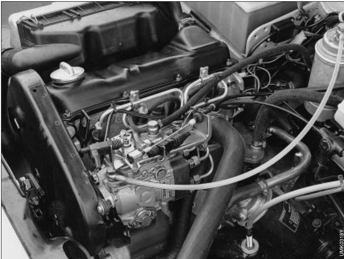
Fig. 2: VE distributor pump fitted to a 4-cylinder diesel engine
