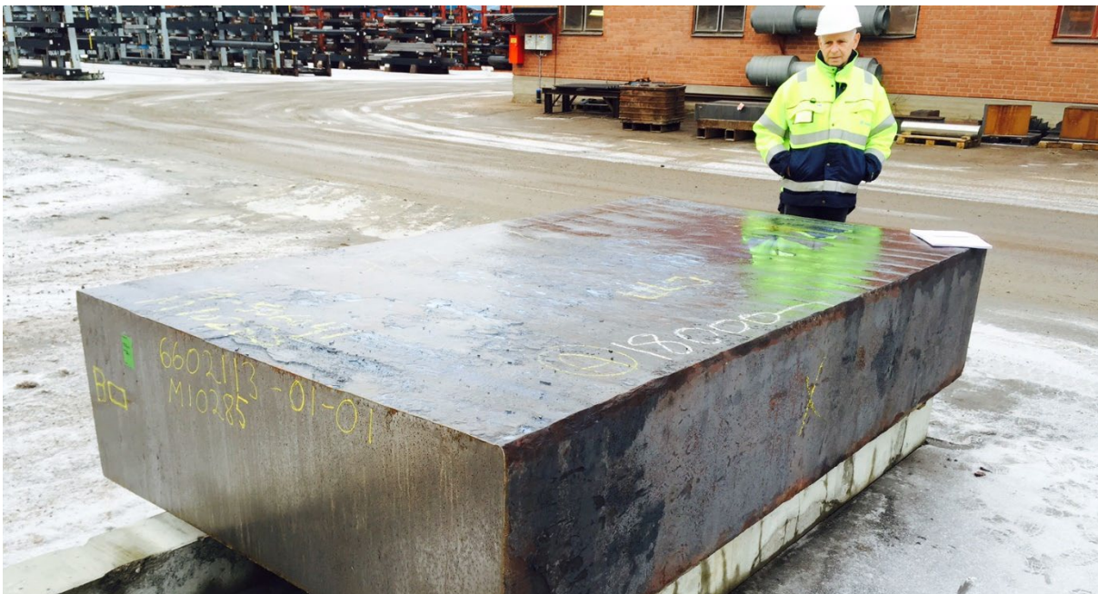
Figure 8 shows just how big some special sizes of Dievar can be manufactured
