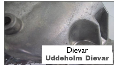
Figure 9 shows a customer case of Dievar and ESR H13 in production with heat checking as the concern
