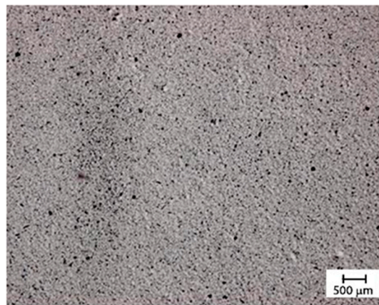
Figure 13. Optical microscopy of the dispersion obtained with the calendar with a distance between the rollers of 0.25 mm.
