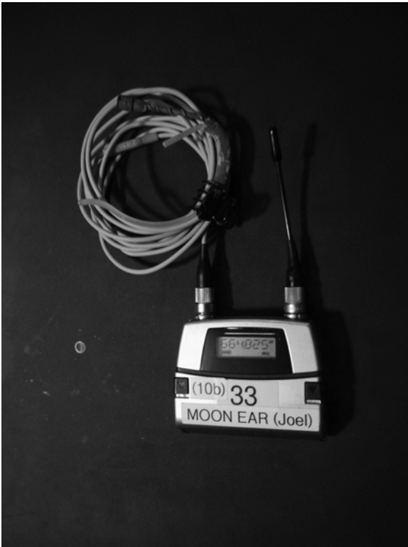
Figure 3.4. This shows the normal method of wrapping the mic to prepare it for delivery to the actors.
