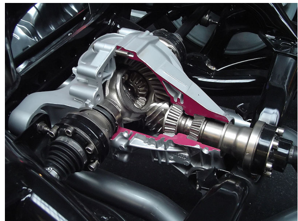
A cutaway view of an automotive final drive unit which contains the differential
