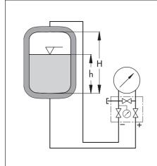
Fig. 2 · Set-up for liquid level measurement. The example shows the standard set-up in a cryogenic application.
