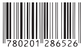
FIGURE 31.25 ▲ A product code is read by laser light that reflects from the bar pattern and is converted to an electrical signal that is fed into a computer. The signal is high when light is reflected from the white spaces and low when reflected from a dark bar.
