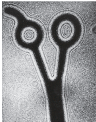
FIGURE 31.8 ▲ Diffraction fringes around the scissors are evident in the shadows of laser light, which is of a single frequency.
