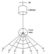
Fig. 2 The spectrum by diffraction grating
