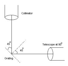
Fig. 1 Normal position of the diffraction grating
