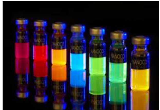
Diagram of a Quantum Dot and vials containing quantum dots produced on an industrial scale. The quantum dots show fluorescent emission peak at different wavelengths depending on their size.
