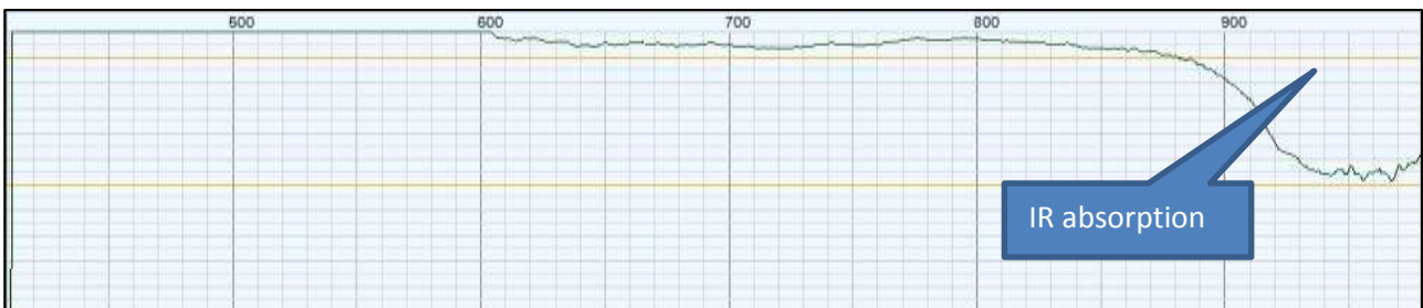
Water absorption (transmission) spectrum. Water absorbs from near IR
