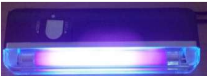
Wood lamp – UV emission at 370nm with tiny visible "tail" beyond 380nm
