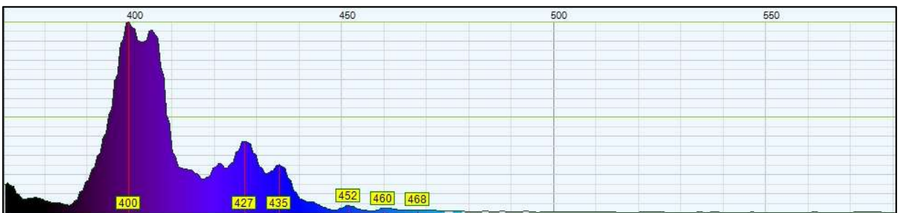
Plasma from high voltage arc – great emission of UV radiation
