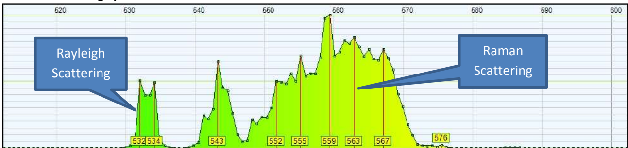
Raman scattering spectrum of ethanol 95% - Excitation 532nm laser
