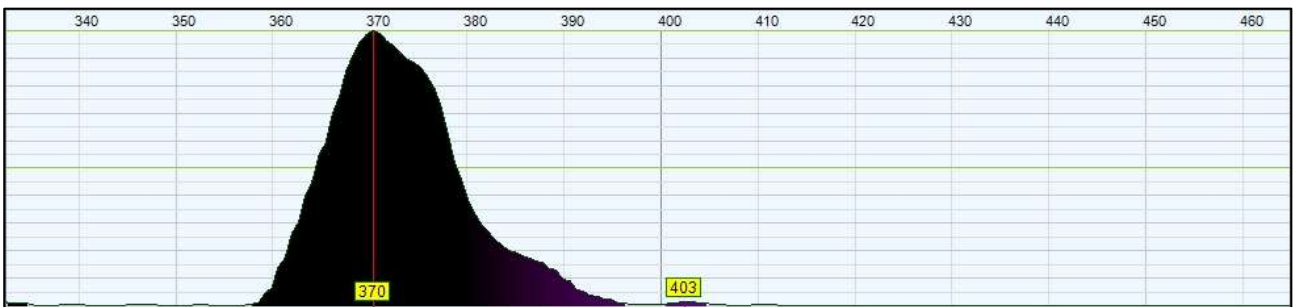
Wood lamp – UV emission at 370nm with tiny visible "tail" beyond 380nm
