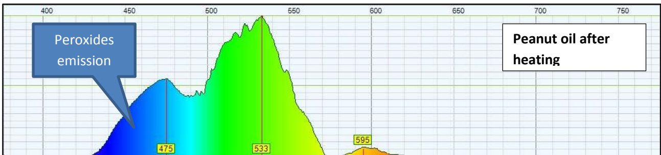
Fluorescence spectrum of peanut oil subjected to heating (thermal degradation) excited by UV emission We note the increase in the intensity of fluorescence at 470nm - 530nm due to thermal degradation of fatty acids and the consequent production of peroxides. The chlorophyll fluorescence has virtually disappeared because the chlorophyll itself has been degraded by heating
