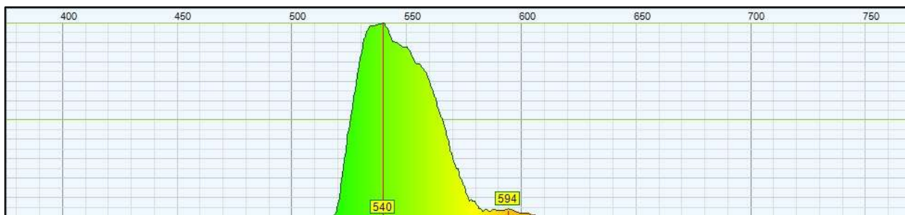
Fluorescence spectrum of tetraphenyl naphthacene (from glowstick) excited by UV emission at 405nm
