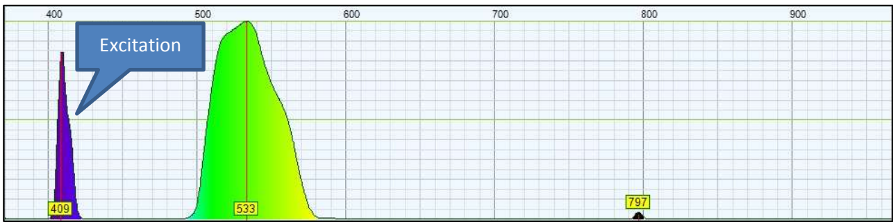
Fluorescence spectrum of uranium glass excited by UV emission
