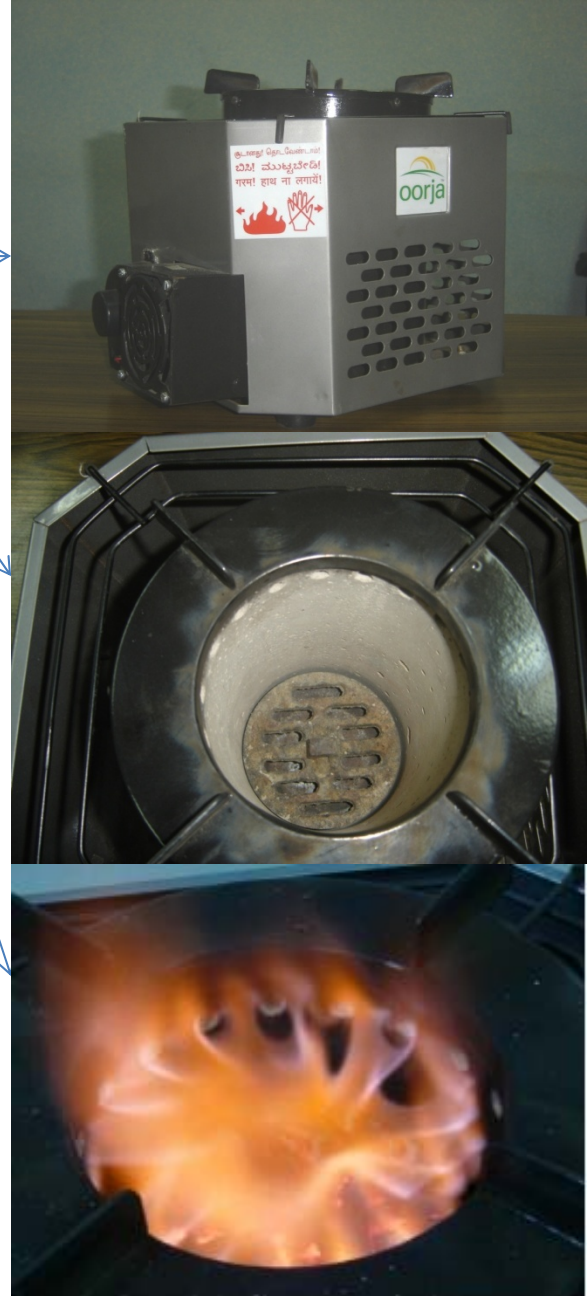
Clean combustion of "producer gas"
