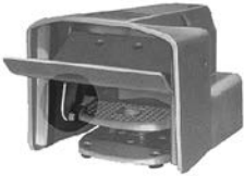
AW124 Type AW Fully Shielded Foot Switch with Oversized Pedal Shield, Side Shields and Safety Door. The Safety Door is interlocked with the pedal to prevent operation due to shock or vibration. It prevents accidental pedal operation by requiring a simple but intentional motion to lift the door before inserting the foot.
