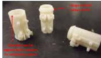
3 individual Biodigits, each with 4 connectors for fluid lines. The connectors can be placed anywhere on the chamber. Here, 2 stick straight out and 2 are turned so that tubing can run along the finger.
