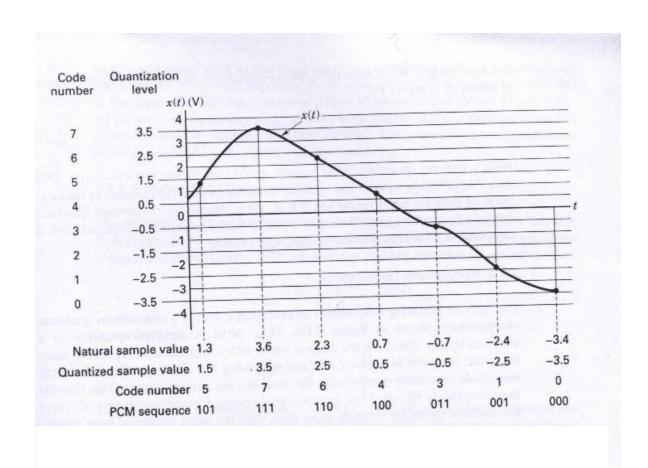
From the above figure each sample of analog signal is assigned to the quantization level closest to the value of the sample. Beneath the analog waveform, x(t), are seen four representations of x(t) as follows:the natural sample value, the quantized sample value, the code numbers, and the PCM sequence.
