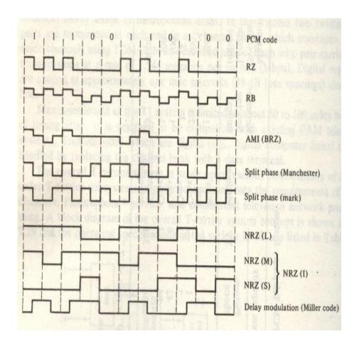
1) Return-to-zero (RZ) method represents a 1 by a change to the level for one-half the bit interval, after which the signal returns to the reference level for the remaining half-bit interval. A 0 is indicated in this method by no change, the signal remaining at the reference level.
