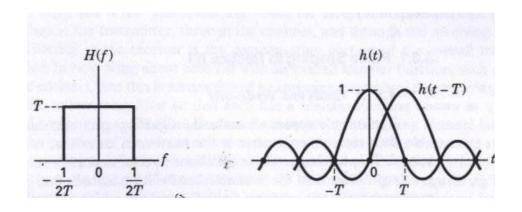
Note that, when H(f) is such an ideal filter with bandwidth 1/2T, its impulse response
