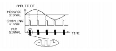
**Pulse-code modulation (PCM)** is sampling the voltage of an analog signal and converting each sample into an 8-bit serial digital code.
