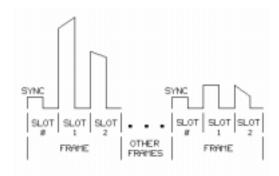
The PAM-TDM receiver also needs synchronization information to locate the time slots. The transmitter tags the beginning of each frame with a synchronization signal. The receiver uses the synchronization tag and the time slot assignment to identify each of the PAM signals.
