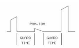
The space between the PAM-TDM pulses is called **guard time**. The guard time prevents interference between adjacent pulses.
