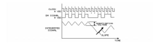
The **quantization voltage** is the amplitude of the integrated signal for one lock (sampling) period. The sampling rate and integrator slope determine the quantization voltage, which affects the quantization errors.
