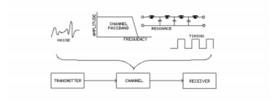
Matching transmitter signal characteristics to channel characteristics minimizes channel effects.
