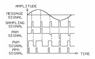
Pulse modulation produces discontinuous pulses that represent **amplitude samples** of the **analog message signal**
