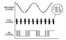
Like PCM, **delta modulation (DM)** is a digital encoding process. PCM converts each message-signal amplitude-sample into an 8-bit code. DM converts the change in the message-signal amplitude to a 1-bit code: logic 1 for an increase, and logic 0 for a decrease.
