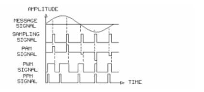
PAM, PWM, and PPM are pulse signals that represent the analog signal by a change in pulse amplitude, width, or position.
