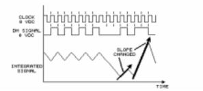
When the quantization errors are detected, the slope of the feedback integrator output is increased or decreased to reduce the errors. CVSD is widely accepted as being potentially a very technically attractive method of digital transmission. The dynamic input signal range of a delta modulation system is limited by slope overload and quantization noise. This dynamic input range can be increased by **companding**.
