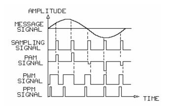
There are different methods for pulse modulating a signal. Each method gets its name from the way pulses are varied to represent the message signal. Two common types of pulse modulation include pulse-amplitude modulation (PAM) and **pulse-time modulation (PTM)**. Two types of PTM are **pulse-width modulation (PWM)pulse-position modulation (PPM)**. In PTM, the timing of the pulse is the variable, not the amplitude as in PAM.
