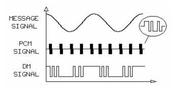
Pulse-code modulation (PCM) is a process that produces a binary code, usually 8 bits, for each amplitude sample. PCM signals are binary encoded PAM signals. Delta modulation (DM) is a process that produces a 1-bit code, which indicates an increase or decrease in the message signal's amplitude.
