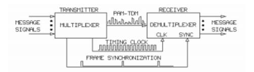
The transmitter **interleaves**PAM pulses into the TDM channel and provides timing and frame **synchronization** information for the receiver. The receiver uses a timing clock to identify when the PAM pulses are valid. Synchronization aligns the receiver with the transmitted TDM frames.
