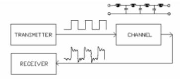
The channel can contain reactances that will oscillate. The oscillations cause **ringing** at the channel's output.
