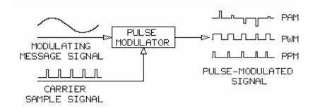
In pulse modulation, the message signal is the **modulating signal**; and the sample signal is the **carrier signal**. The message signal modulates the sample signal to produce the pulse modulated signal (PAM, PWM, or PPM).
