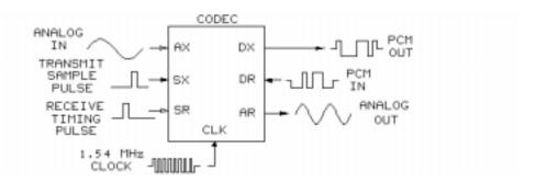
A **CODEC** (encoder/decoder) IC performs the analog-to-digital conversion (encoding) for the transmission of PCM signals.
