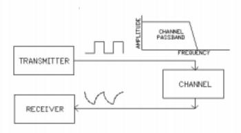
A channel with a poor high-frequency characteristic affects the pulse rise and fall times. Limited bandwidth increases the time a pulse needs to attain the amplitude required by the receiver.
