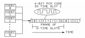
**Time-division multiplexing (TDM)** is the process by which many channels of PCM signals representing different messages are transmitted over the same line.
