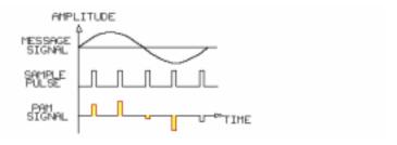
To demodulate the PAM signal into the original message signal, the PAM signal must be formed by a sample pulse frequency ( $f_s$ ) greater than two times the maximum message signal frequency ( $f_m$ ).
