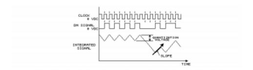
The DM transmitter described produces **linear DM**, because it has a fixed slope. **Continuously variable slope delta modulation (CVSD)** is another DM method. CVSD monitors the signal for signs of distortion.
