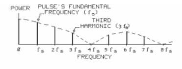
The frequency spectrum of a PAM signal is shown. The message signal frequency  $(f_m)$  is present in addition to a number of **replicas**; only three are shown.
