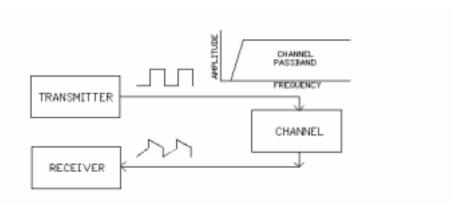
A channel with a poor low-frequency characteristic can affect the top and bottom of a pulse. The pulses do not maintain a stable voltage level, making them difficult to detect.
