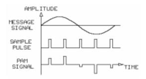
In PAM, the blank time space between the transmitted PAM amplitude pulses is uniform because the sampling frequency is constant. PAM signals from other message signals can be inserted into this blank time space for the transmission of **multiplexed signals**.
