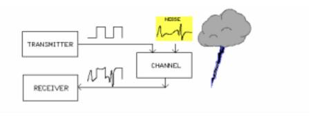
Noise is an interference signal which the channel adds to the transmitter signal. The noise signal affects the amplitude and possibly the logic state of the receiver's input pulses.
