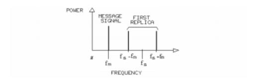
If the first replica is removed during demodulation, all the other replicas are also removed.
