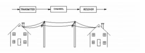
The channel is a path used to pass signals between the transmitter and receiver. A **digital communications channel** carries digital signals (pulses) which represent the message being transferred. A digital channel can use any **media** to carry the pulses including: twisted wire, fiber optics, or coaxial cable. All channels distort the signals they carry.
