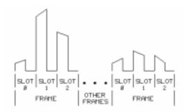
The TDM channel is divided into time periods called **time slots**. Time slots have a fixed order that repeats once each **frame**. Each message signal is assigned to one of the time slots. As the frame repeats, one PAM sample from each message signal is placed in its assigned time slot.
