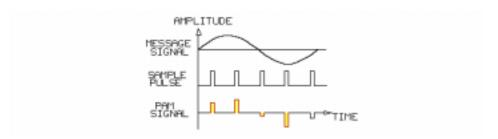
Instead of transmitting the analog waveform, it is possible to transmit pulses that represent the message signal's waveform.
