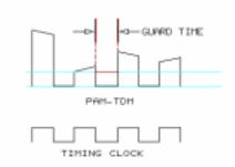
A timing clock can be extracted using the PAM pulses and the guard time spaces. A minimum PAM pulse height, or **pedestal**, ensures that a stable timing clock can be recovered from the PAM-TDM. The receiver uses the timing clock to identify when the PAM pulses are valid.
