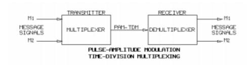
**Time-division multiplexing (TDM)** simultaneously sends multiple message signals over a single channel. The transmitter, or **multiplexer**, combines the message signals into a single pulse-amplitude modulated (PAM) TDM signal. The receiver, or **demultiplexer**, separates the PAM-TDM signal back into message signals.
