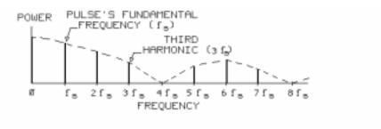
The frequency domain of a pulse signal is shown.
