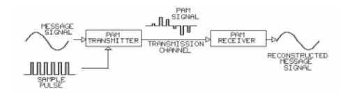
The PAM signal, rather than the analog message signal, is transmitted to a receiver. The PAM receiver demodulates (reconstructs or recovers) the PAM signal into the original analog message signal.
