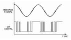
DM can be considered as a 1-bit differential pulse-code modulation system. A logic 0 means that the message signal's amplitude is decreasing. A logic 1 means that the message signal's amplitude is increasing.
