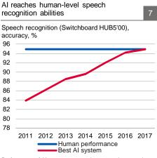
Performance of AI systems on a task to recognize speech from phone call audio; Word Error Rate (WER) of trained speech recognition systems on Switchboard Hub5'00 data. Sources: Artifical Intelligence Index, Electronic Frontier Foundation, AI Progress Metrics
