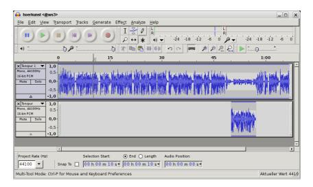
Each track has a small triangle symbol at the bottom of the label (heading), click on it to reduce or enlarge the view on the sound track .
