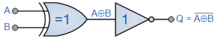
2-input "Ex-OR" gate plus a "NOT" gate
