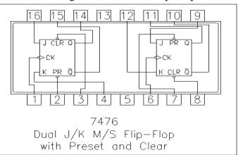
Pin diagram of JK M/S Flip Flop
