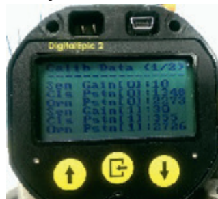
FIGURE 102 Viewing calibration data sub-menu
