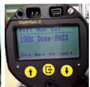
FIGURE 60 Performing manual calibration - open position
