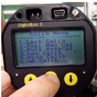
FIGURE 63 Accessing low calibration
