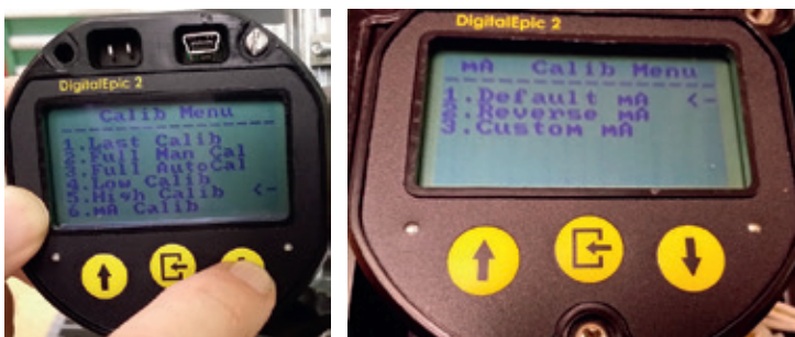
FIGURE 67 Accessing mA calibration
