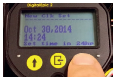
FIGURE 43 Configuring clock - date setup
