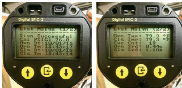
FIGURE 84 Viewing maintenance signature data
