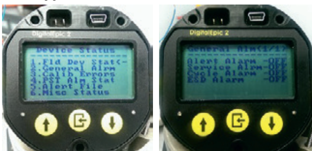
FIGURE 93 Accessing general alarm status menu
