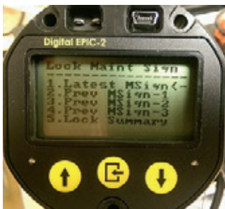
FIGURE 85 Locking/unlocking maintenance signatures menu
