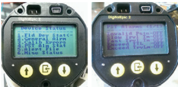
FIGURE 96 Accessing alert file menu
