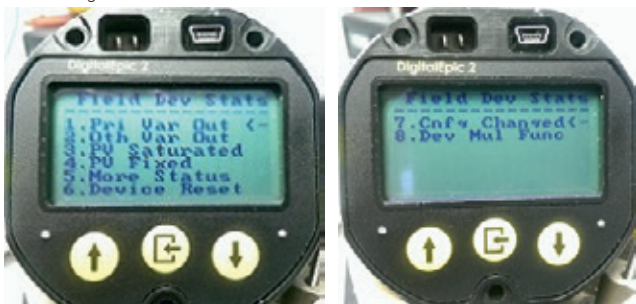
FIGURE 91 Accessing field device status sub-menu
