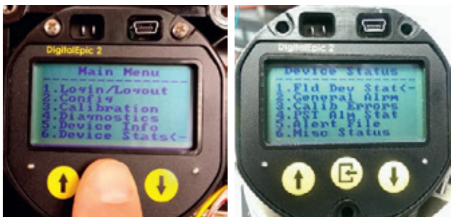
FIGURE 90 Navigating to device status menu
