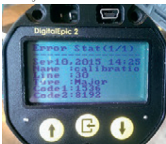
FIGURE 99 Viewing error status
