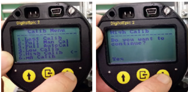
FIGURE 65 Accessing high calibration
