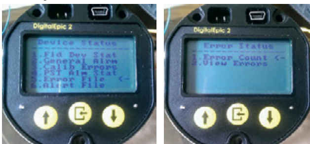
FIGURE 99 Viewing error status
