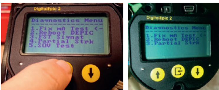
FIGURE 75 Fixed mA test
