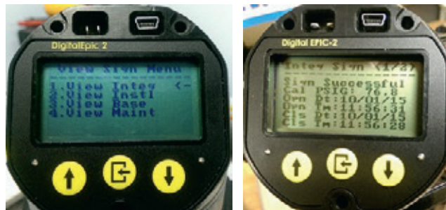
FIGURE 79 Viewing integrator signature data
