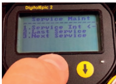
FIGURE 53 Accessing service configuration menu
