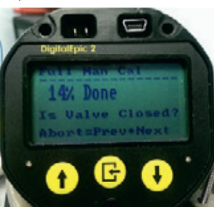
FIGURE 59 Performing manual calibration - close position
