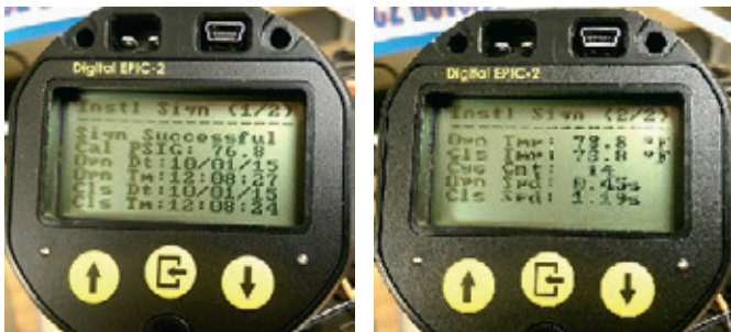
FIGURE 81 Viewing installer signature data
