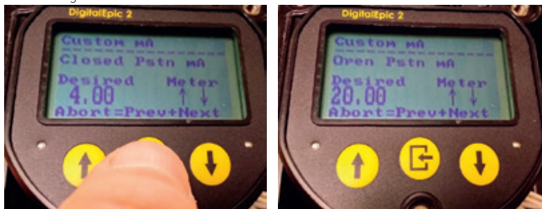
FIGURE 71 Performing custom mA calibration
