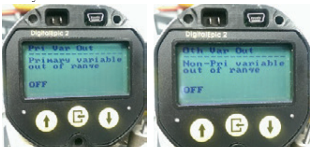
FIGURE 92 Viewing status bits in field device status
