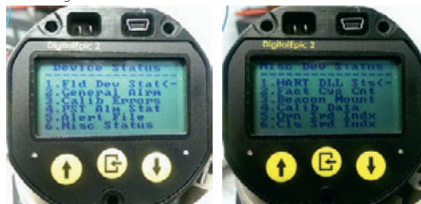
FIGURE 100 Accessing miscellaneous device status
