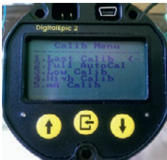
FIGURE 61 Accessing full auto calibration
