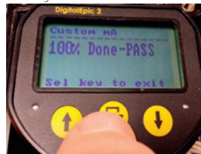
FIGURE 72 Finishing custom mA calibration
