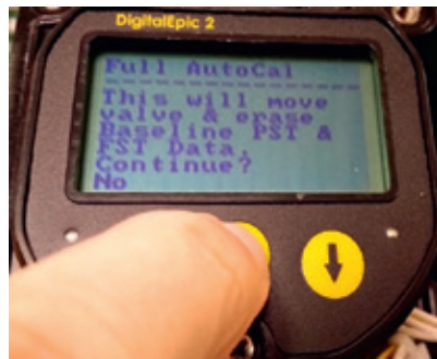
FIGURE 62 Performing auto calibration
