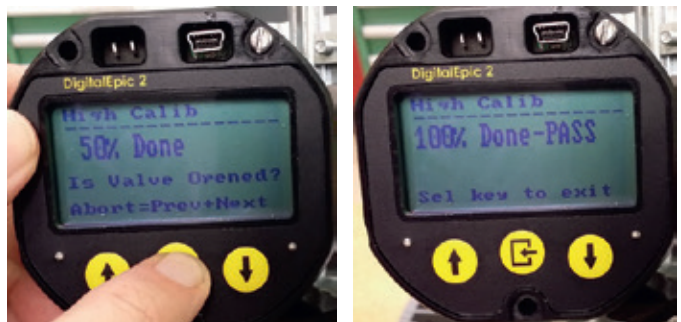
FIGURE 66 Performing high calibration
