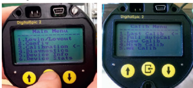
FIGURE 56 Accessing calibration menu
