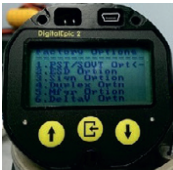
FIGURE 39 Performing factory defaults
