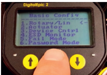
FIGURE 44 Accessing basic configuration menu
