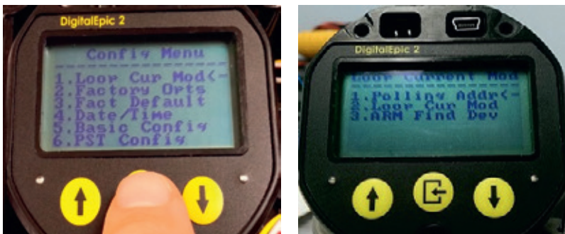
FIGURE 35 Navigating to loop current mode menu
