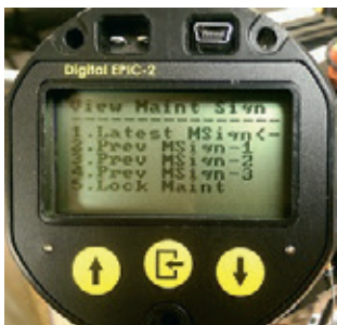
FIGURE 83 Accessing view maintenance signature menu
