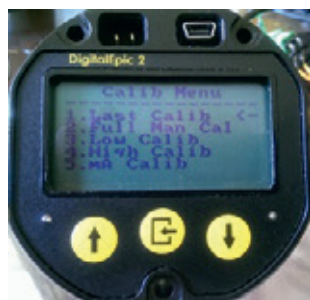
FIGURE 58 Full manual calibration
