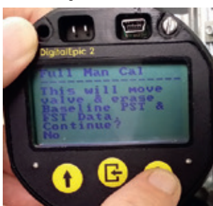
FIGURE 59 Performing manual calibration - close position
