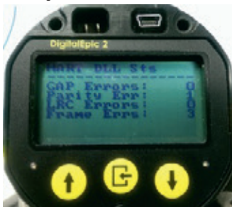
FIGURE 101 Viewing HART DLL statistics
