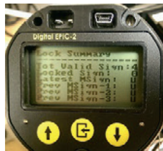
FIGURE 85 Locking/unlocking maintenance signatures menu
