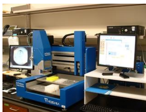
Automated Crystallization Systems: Hamilton (left) and Phoenix crystallizers (right)
