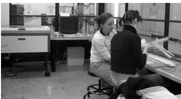
Fig. 30. Students building a model with laser cut parts; laser cutter in the background. (Christine Gaspar and Marlene Kuhn)
