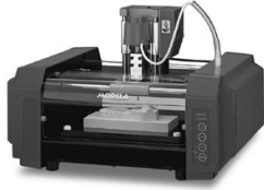
Fig. 5. Roland Modela MDX-20 desktop milling machine.
