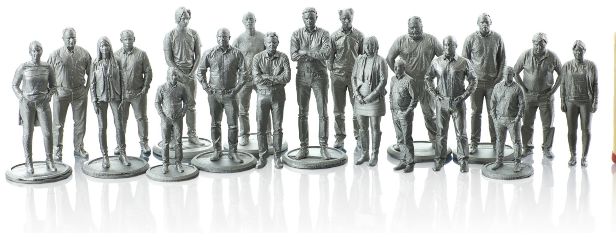
Fig. 11 In 2017, in a demonstration of the high resolution achievable using its technology, Digital Metal produced a batch of figurines representing a part of its team. Standing at roughly the same height as a matchstick, the figurines have toured with Digital Metal to some of the key AM industry events
