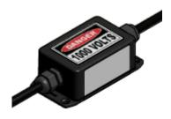
The shunt is used with the inductive couplers to enhance the quality and strength of the BPL signal. It is installed directly across two phases of the power line, and provides a return path for the BPL signal
