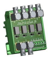
The BPL signal switcher allows a single BPLM to be permanently connected to a number of cables, and allows users to select which cable or cables the BPL signal is coupled onto. This can be used in a distribution board, for example, where there are many outlets, and equipment can be connected to any of them. Signal switchers can be daisy chained.
