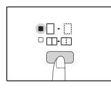
To select the "EDGE + CENTRE ERASE" mode, press the [ERASE] key ( [] • [] / []] • []] ) until both the EDGE (□ · □) and CENTRE up.
