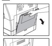
When feeding large paper such as B4 and A3 (8-1/2" x 14" and 11" x 17"), pull out the bypass tray extension.
