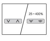
Press the [PRESET RATIO] selector keys  $( \ varsim , \ warrow )$  to select a ratio close to the desired ratio, and then press the [Zoom] keys (  $\ varsim , \ varsim )$  to adjust the ratio in increments of 1%. The ratio appears in the display.
