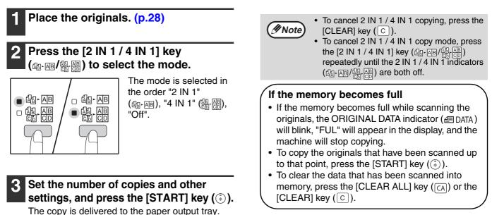
Setting the layout pattern You can select the layout pattern for copying 2 original pages or 4 original pages onto one sheet of paper. The available layout patterns are shown on the first page of this section.
