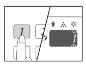
To enable the setting, press [1] key. To disable the setting, press [0] key. The factory default setting is "0". The entered number appears in the first digit of the number of copies display.
