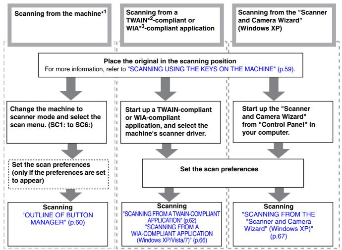
\*<sup>1</sup> To scan using the machine's operation panel, you must first install Button Manager and establish the appropriate settings in the Control Panel. For details, see "SETTING UP BUTTON MANAGER" (p.12).
