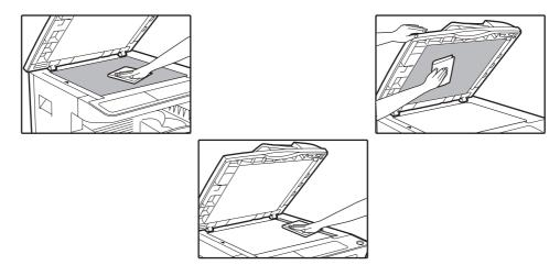
Stains or dirt on the document glass/SPF/RSPF will also be copied. Wipe the document glass, underside of the document cover/SPF/RSPF and the scanning window on the document glass with a soft, clean cloth. If necessary, dampen the cloth with water. Do not use thinner, benzene, or similar volatile cleaning agents.
