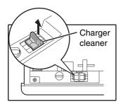
5 Set the charger cleaner onto the transfer charger and gently slide the cleaner in the direction indicated by the arrow two or three times.
