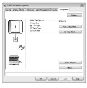
**IDENTIFY and SET UP:** To automatically configure the settings based on the detected machine status, click the "Auto Configuration" button.
