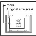
Place the original face down on the document glass. Align the edge of the original with the original size scale, to be centred with the centring mark (>).
