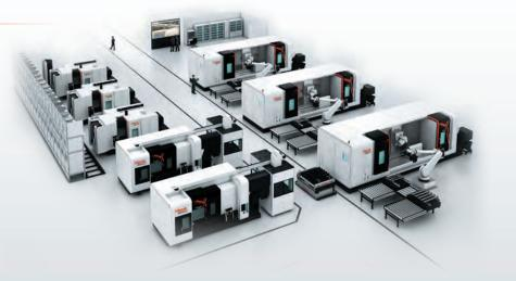
The MTConnect open communications protocol, along with process support software, monitors and harvests data from all production floor machines, cells, devices and processes. With PCs, smartphones and tablets, management and manufacturing teams access real-time data for improved production efficiency and responsiveness. Customers can achieve these same results in their shops, and Mazak not only makes it possible: It shows customers the way.
