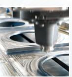
Friction Stir Welding (FSW)
