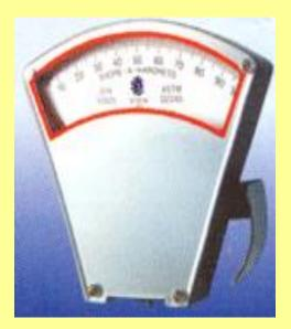
The Shore Hardness is defined as the resistance to penetration by an indentor of specified shape under a defined load.
