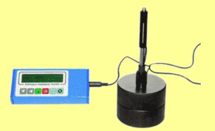
The Portable Hardness Tester an advanced pocketable hardness tester distinguished by its high accuracy, wide measuring range, simplicity of operation & above all it is a really portable instrument operating on three pencil cells of size AA. It is suitable for testing the hardness of many materials & finds applications for hardness testing in many areas of industry.
