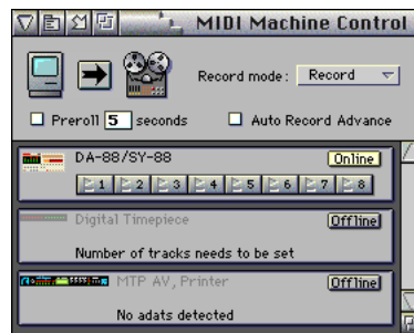
Figure 9-8: Setting up control of the DA-88/SY-88 in Performer. Take the Digital Timepiece and MIDI Timepiece AV off line, and bring the DA-88/SY-88 on line.
