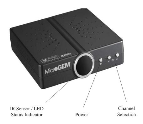
\* Power LED- When the LED is lit red, the unit is in STAND-BY mode. Press the "POWER" button to wake the unit. When the unit is active, the LED will light green.
