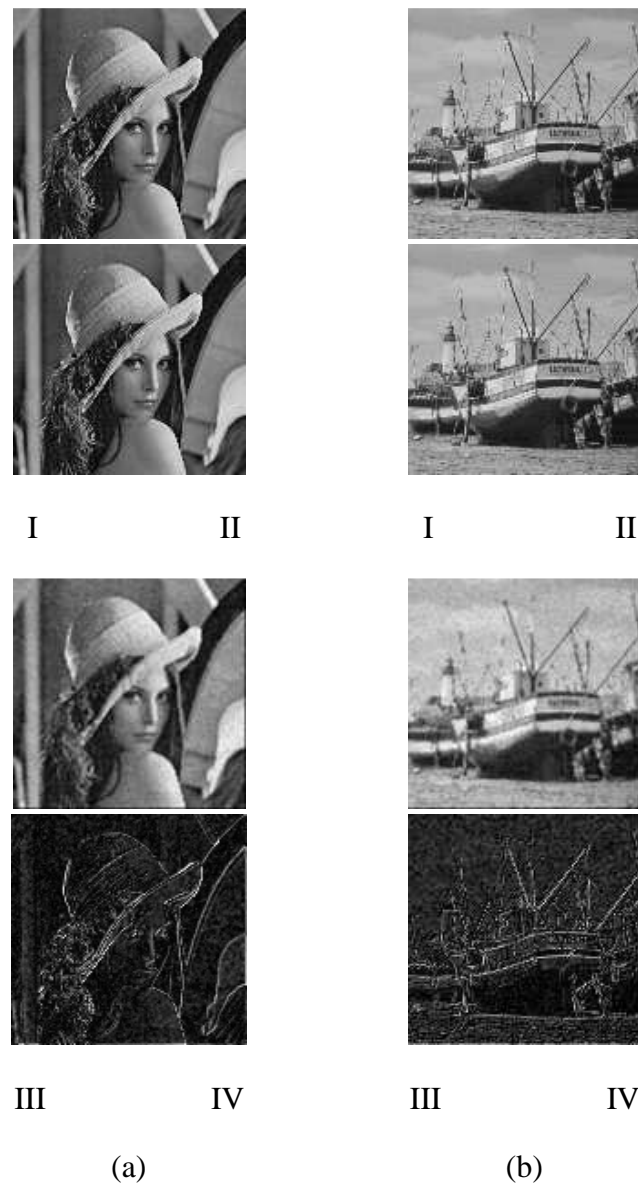
Fig.3.5 Watermark Structuring: I.original image, II. watermarked image, III. attack sequence B applied on watermarked image, and IV. scaled difference image of I and II for (a) Lena image and (b) Boat image.
