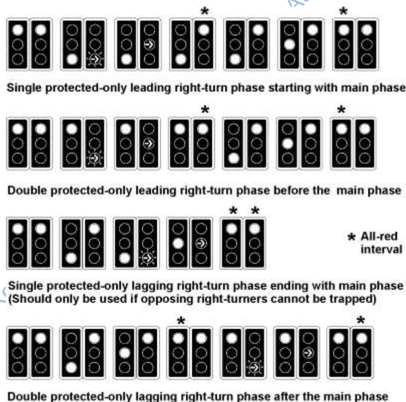
Figure 3.5b: Traffic signal sequence for protected-only right-turn phases using the S1 and S1R signal faces in conjunction with ST5 and ST2 traffic signal arrow signs.
