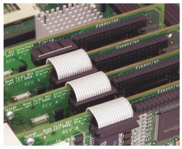
Figure 8: Timing Ports Example
