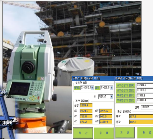
3D measurement software 소프트웨어 (Instant access to measured data using Mobile and PDA)
