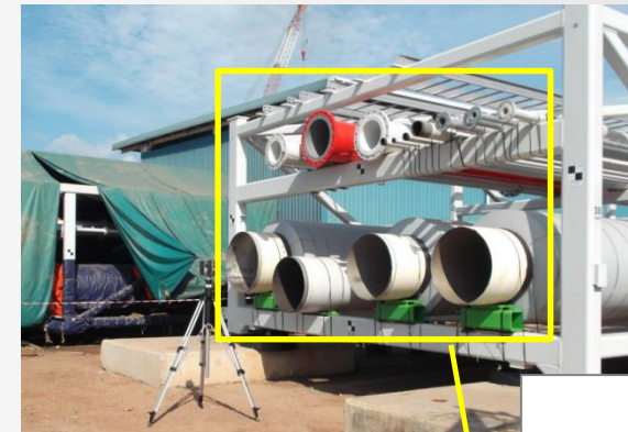
Pipe Rack -3D Laser Scanning (for Pipe Rack Alignment Check)
