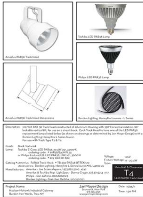
Figure E.5. Track head T4, using LED PAR38 lamp.
