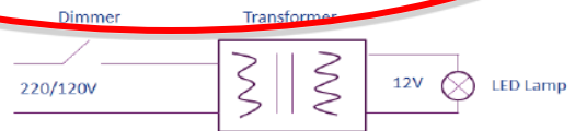
Figure G.4. GE 7W LED MR16 dimmer compatibility guidance, showing the trailing edge (reverse phase, ELV) dimmer is likely to work best with this LED lamp installed in an electronic transformer track head. (Source: http://www.gelighting.com/LightingWeb/na/images/led-replacement-lamps-dimmer-compatibility-table.pdf .)
