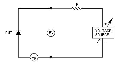
NOTE: The ammeter shall present essentially a short-circuit to the terminals between which the current is being measured or the voltmeter readings shall be corrected for the drop across the ammeter.
