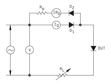
NOTE: The reverse leakage current at each device  $D_1$  and  $D_2$  shall be less than .05 percent of the maximum allowable specified leakage current of the DUT. In other respects, the devices  $D_1$  and  $D_2$  should be of the same type as the DUT.
