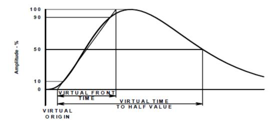
FIGURE 4066-6. Standard current impluse waveshape.
