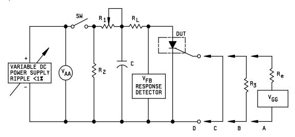
FIGURE 4231-1. Test circuit for exponential rate of voltage rise.
