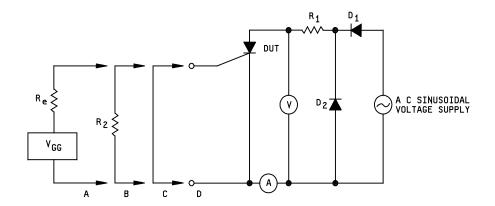
NOTE: The ammeter shall present essentially a short-circuit to the terminals between which the current is being measured or the voltmeter readings shall be corrected for the drop across the ammeter.
