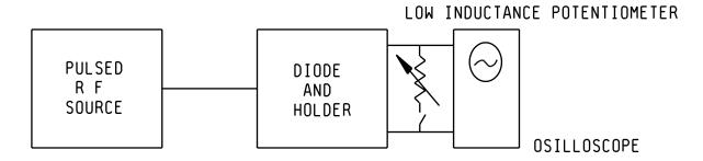
FIGURE 4131-3. Pulsed RF method.
