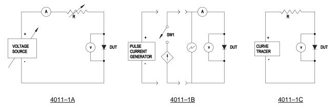
FIGURE 4011-1. Test circuits for forward voltage.
