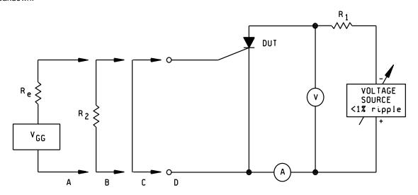
NOTE: The ammeter shall present essentially a short-circuit to the terminals between which the current is being measured or the readings shall be corrected for the drop across the ammeter.
