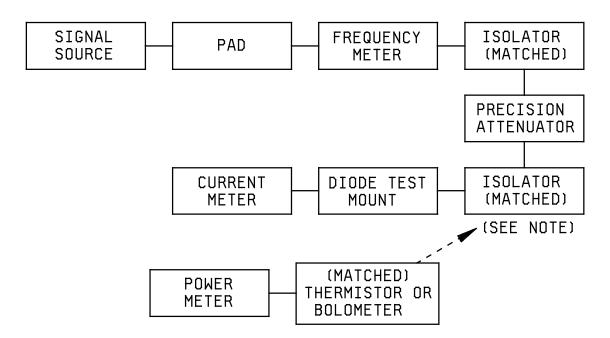
FIGURE 4111-1. Test setup for figure of merit measurement.
