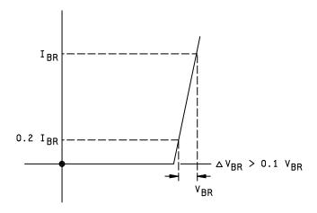
The slope shall be less than 10 percent of  $V_{BR}$  when viewed between 20 percent to 100 percent of the specified  $I_{BR}$  or  $I_{Z}$ . Low voltage zeners below 5.5 volts are in exception to this requirement also, or other devices, as may be specified.
