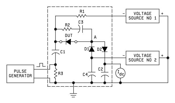
FIGURE 4061-1. Test circuit for stored charge.
