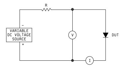
NOTE: To assure accurate measurement of reverse leakage current, the voltage drop across the ammeter shall be subtracted from the measured value of reverse voltage. Resistor (R) shall be chosen to limit the current flow in the event the device goes into reverse breakdown.
