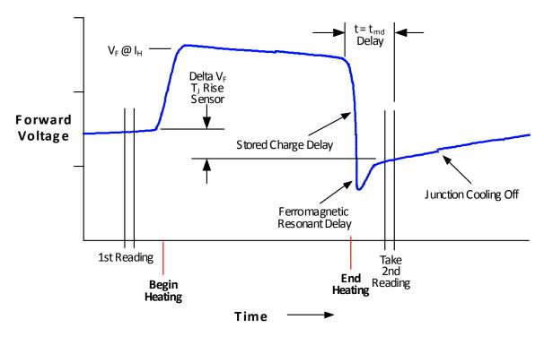
FIGURE 4081-A1. Analysis of theta test.
