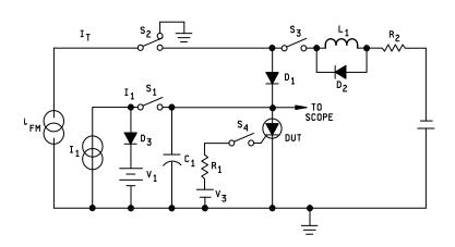
NOTE: The simplified circuit diagram on figure 4224–2 illustrates the operating principles of a circuit used to generate the waveforms illustrated on figure 4224–1. For purposes of clarity, the circuit diagram utilizes current generators, ideal switches, and no provision for repetitive test cycles.
