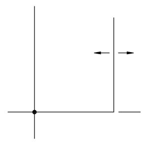
The vertical component of the trace should remain stable in the horizontal axis. An undesirable drift is defined as greater than a 10 percent increase or 2 percent decrease in actual breakdown voltage up to 1,500 volts. If over 1,500 volts, the allowable drift should be separately specified.
