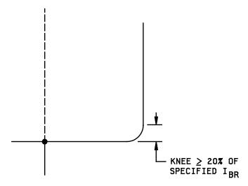
The knee area is the area in which the trace transitions from the horizontal to the vertical. Unless otherwise specified, this area should not require more than 10 percent of the total horizontal voltage component being viewed, or more than 20 percent of the specified  $I_{BR}$ . Not applicable to signal diodes, low voltage zeners, fast, ultrafast, and Schottky rectifiers or low voltage zeners  $\leq$  10 volts.
