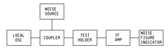
FIGURE 4126-1. Test setup for overall noise figure.
