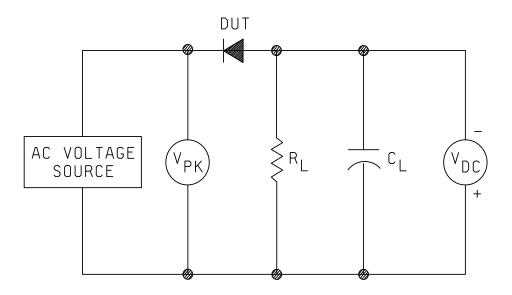
NOTE: The voltmeter shall have a high impedance as compared with the load circuit of R<sub>L</sub> and C<sub>L</sub>.
