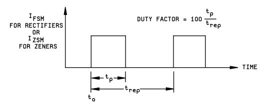
FIGURE 4066-4. Rectangular current pulse waveforms.
