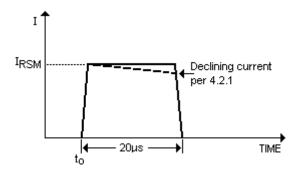
FIGURE 4065-2. Rectangular 20µs Current Pulse Waveform.
