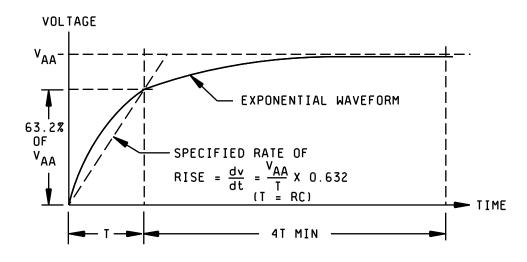
FIGURE 4231-2. Waveforms across the DUT.
