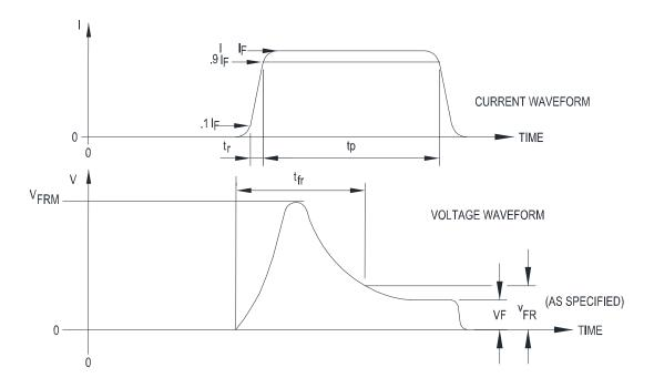
FIGURE 4026-2. Input forward current pulse and output voltage waveforms.
