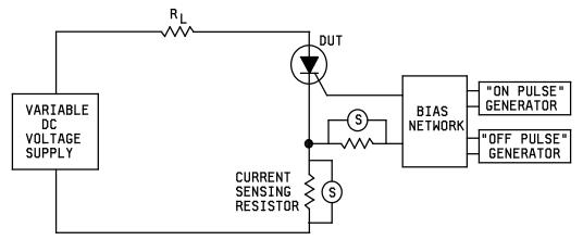
FIGURE 4225-1. Gate turn-off test circuit.
