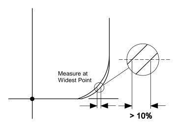
For soft knee diodes including signal diodes, low voltage zeners, and altered junction fast, superfast and ultrafast rectifiers, the region at the knee may display a secondary trace no more than 10 percent of the total voltage of the DUT (see detail).
