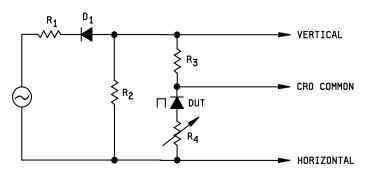
FIGURE 4321-1. Test circuit for negative resistance, short-circuit stable method.
