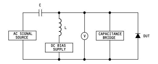
NOTE: Both dc bias and ac signal sources may be incorporated in the capacitance bridge. The dc bias source should be properly isolated, preferably with an inductance L in series and have negligible capacitance compared to the DUT. The reactance of C must be negligible compared to the reactance of the DUT, at the frequency of measurement. Impedance of voltmeter should be at least 10 times that of the DUT.
