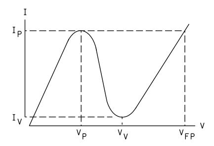
FIGURE 4306-3. Typical tunnel diode forward characteristic.
