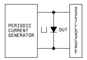
FIGURE 4331-1. Test circuit for switching time.
