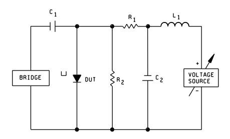
FIGURE 4301-1. Test circuit for junction capacitance.
