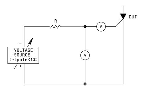
NOTE: The ammeter shall present essentially a short-circuit to the terminals between which the current is being measured or the voltmeter readings shall be corrected for the drop across the ammeter.
