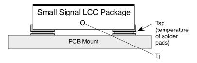
FIGURE 4081-6. Surface-Mount arrangement and Temperature Sensing Location (LCC).
