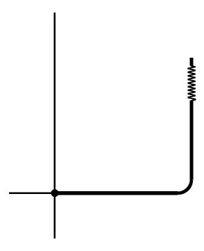
Instability (arcing) appearing at or near the specified  $I_{BR}$  region on the vertical trace (such as may be coincident with visible sparking activity within the device die region) shall not be present. Noise at or near the knee is permissible, such as typically observed on avalanche-zener devices.
