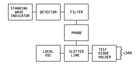
FIGURE 4136-1. Slotted line method.
