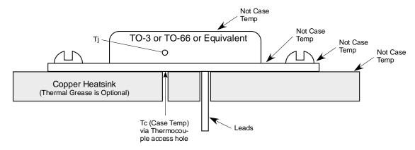
FIGURE 4081-4. Case mounting arrangement. (TO-3 or TO-66).
