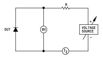
NOTE: The voltmeter being used to measure the terminal voltage should present an open circuit to the terminals across which the voltage is being measured.
