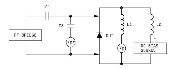
NOTE: The impedance of C1, C2, and L1, L2 shall be small and large, respectively, compared to the DUT at the frequency of measurement.
