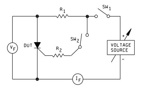
NOTE: When specified, switch SW<sub>1</sub> shall be used to provide pulses of short-duty cycle to minimize device heating. When pulsing techniques are used, other suitable peak-reading techniques shall be used to measure the necessary parameters, and the duty cycle and pulse width shall be specified.
