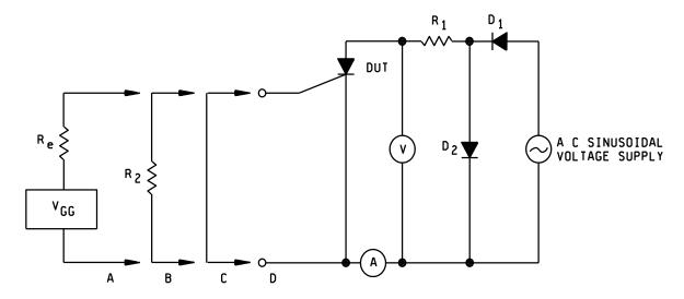
NOTE: The ammeter shall present essentially a short-circuit to the terminals between which the current is being measured or the voltmeter readings shall be corrected for the drop across the ammeter.
