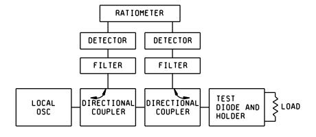
FIGURE 4136-2. Reflectometer method.
