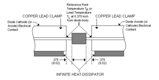
FIGURE 4081-2. Axial-leaded mounting arrangement.
