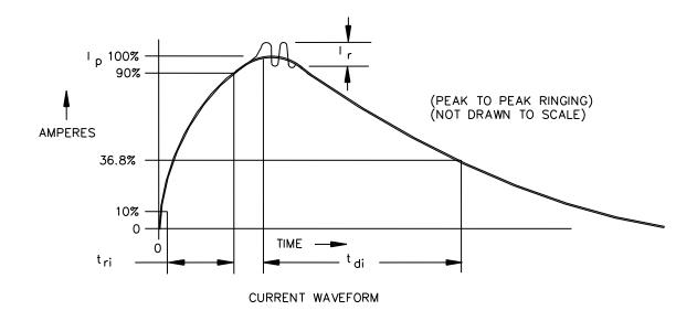
$t_{ri}$  (rise time)-----Less than 10 ns.  $t_{di}$  (delay time)-----150 ±20 ns.
