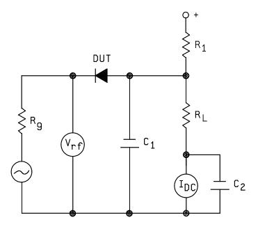
FIGURE 4106-1. Test circuit for detector power efficiency.
