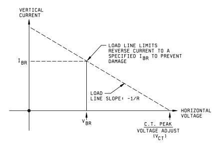
This ideal trace exhibits none of the characteristics described on the figures below. Also, illustrated are the basic curve tracer adjustments and relation for a safe maximum operating current ( $I_{BR}$ ) with the series load resistor (R) versus peak open circuit voltage ( $V_{CT}$ ) and device breakdown voltage ( $V_{BR}$ ).
