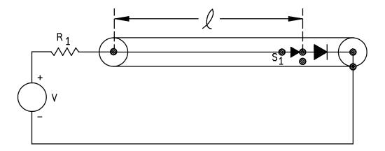
FIGURE 4146-1. Burnout by single pulse.
