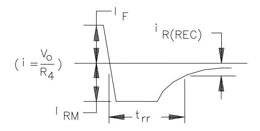
FIGURE 4031-5. Current through DUT (condition B).
