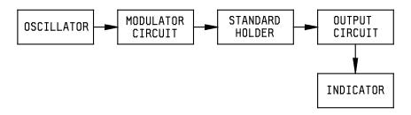
FIGURE 4101-4. Test setup for modulation measurement.
