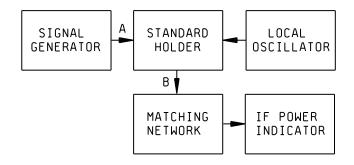
FIGURE 4101-3. Test setup for heterodyne measurement.
