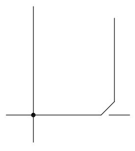
The double break is the area in which the trace transitions from the horizontal to the vertical. Unless otherwise specified, this area should not occupy more than 10 percent of the total horizontal voltage component being viewed, or more than 20 percent of the specified  $I_{BR}$  or  $I_{ZT}$ . This requirement is not applicable to ultrafast or Schottky rectifiers, and low voltage zeners  $\leq$  10 volts.
