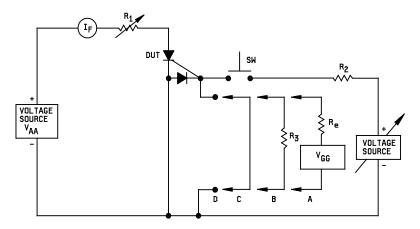
FIGURE 4201-1. Test circuit for holding current.
