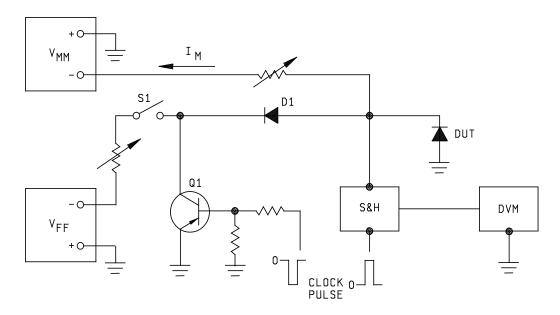
FIGURE 4081-1. Test circuit.
