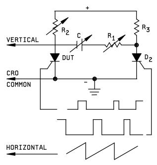
FIGURE 4216-1. Test circuit for pulse response.
