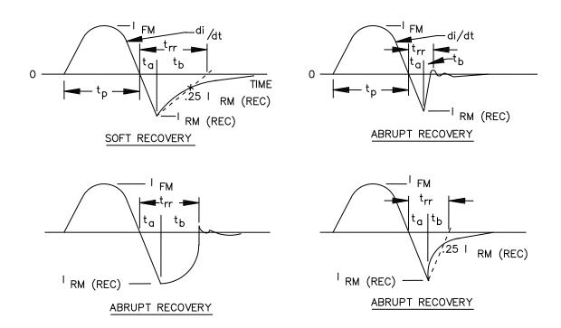
FIGURE 4031–7. <u>Test current waveforms for various types of rectifier diodes under test in the circuit for measuring reverse recovery characteristics.</u>
