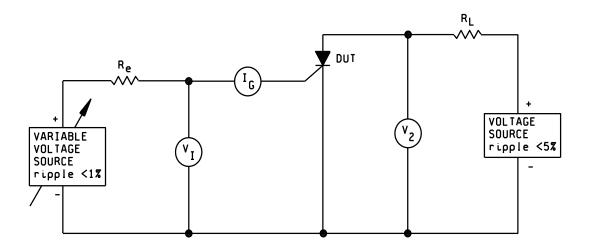
NOTE: The ammeter shall present essentially a short-circuit to the terminals between which the current is being measured or the voltmeter readings shall be corrected for the drop across the ammeter.
