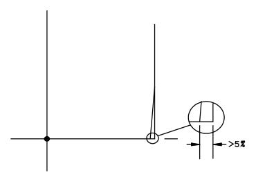
For standard rectifiers and zeners, the region at the knee may display a secondary trace no more than 5 percent of the total voltage of the DUT (see detail).
