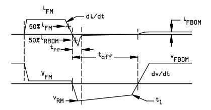
FIGURE 4224-1. Circuit-commutated turn-off time waveforms.
