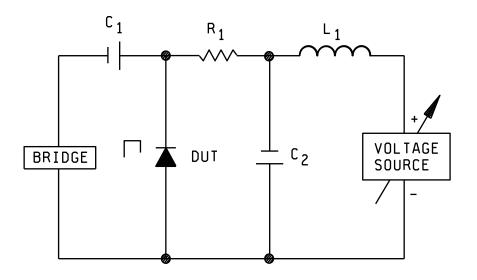
FIGURE 4316-1. Test circuit for series inductance.
