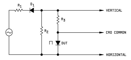
FIGURE 4326-1. Test circuit for series resistance.
