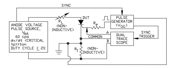
FIGURE 4223-1. Test circuit for gate-controlled turn-on time.
