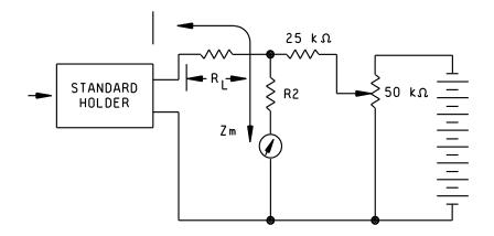
FIGURE 4101-2. Output circuit for the incremental measurement.
