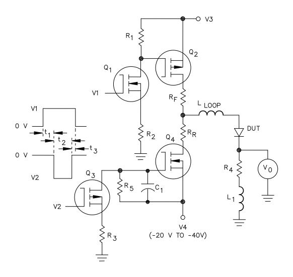
$V_3$  and  $R_F$  control forward current  $I_F$   $V_4$  and  $R_R$  control reverse current  $I_{RM}$   $t_{rr(\text{max})}$  is the longest to be measured.  $t_{rr(\text{min})}$  is the shortest expected.
