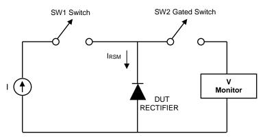
FIGURE 4065-1. Rectangular current pulse test setup.
