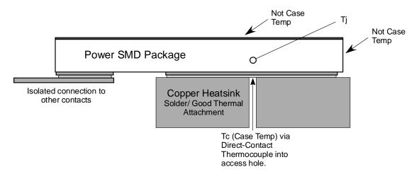
FIGURE 4081-5. Surface-Mount arrangement and Temperature Sensing Location (SMD)
