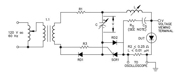
NOTE: Rs and Cs are snubber components, when their use is specified
