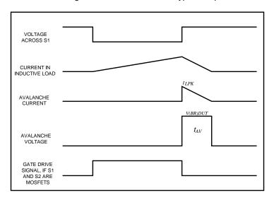
FIGURE 4064-4. Test Circuit 2 response.
