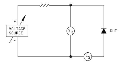
FIGURE 4076-1. Test circuit for saturation current.
