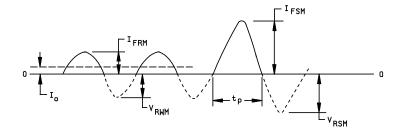
NOTE: Surge current pulse (tp) does not require synchronization with applied baseline ac.
