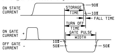
FIGURE 4225-2. Typical gate turn-off circuit waveforms.
