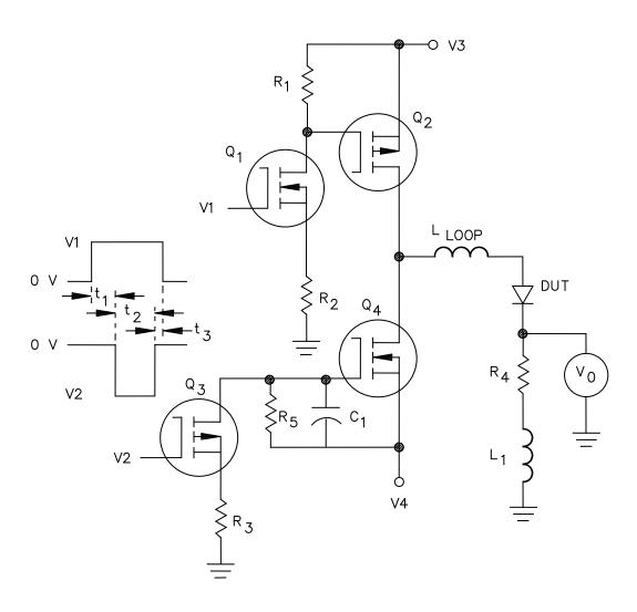
$V_1$  amplitude controls forward current (I<sub>F</sub>).  $V_2$  amplitude controls di/dt.  $t_{a(\text{max})}$  is the longest  $t_a$  to be measured.  $t_{a(\text{min})}$  is the shortest  $t_a$  to be measured.
