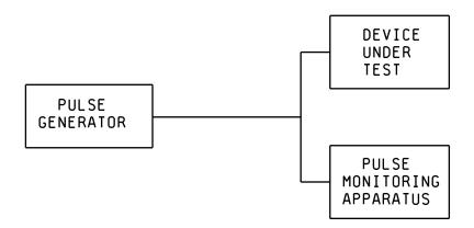
FIGURE 4141-1. Test setup for repetitive pulsing.
