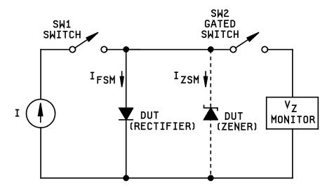
FIGURE 4066-3. Rectangular current pulse test setup.
