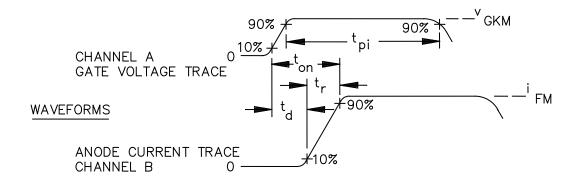
FIGURE 4223-2. Waveforms, gate-controlled turn-on time.
