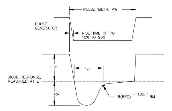
FIGURE 4031-2. Response pulse waveforms for condition A.
