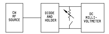
FIGURE 4131-4. Continuous wave RF method.
