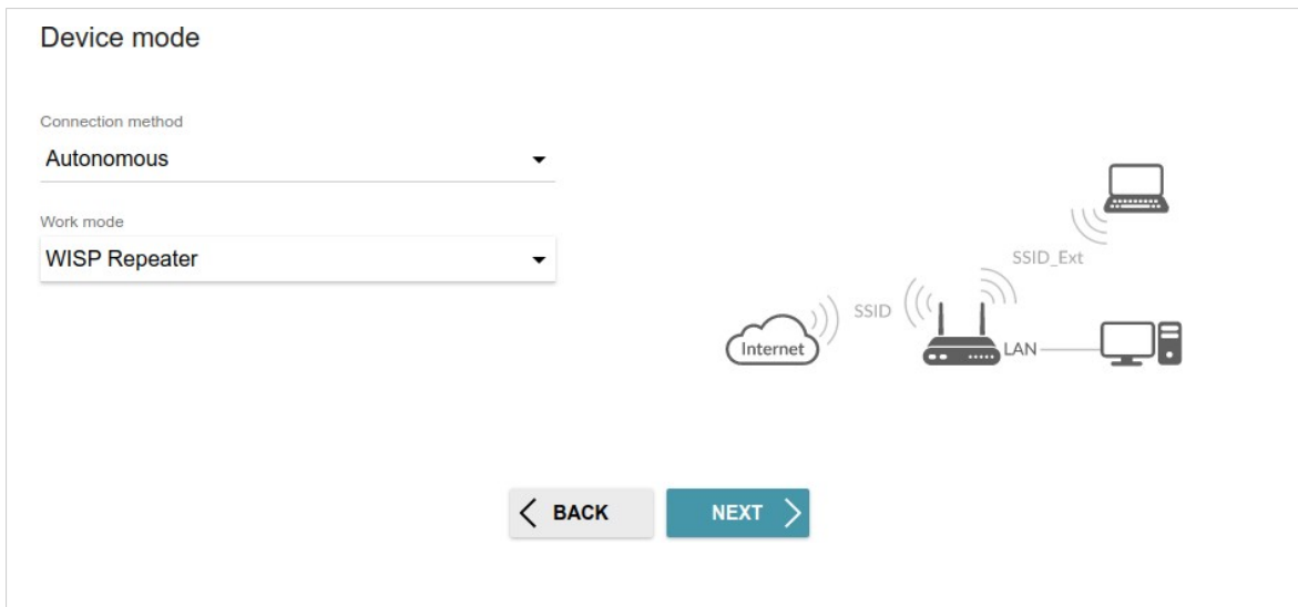
Figure 38. Selecting an operation mode. The WISP Repeater mode.
