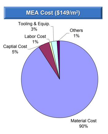
In 2005, the MEA cost was higher due to higher material costs for the membrane (2 mil), electrodes (Pt loading =  $0.75 \text{ mg/cm}^2$ ) and GDL (woven carbon fiber = 30/kg).
