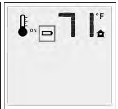
Figure 16: Low Battery Indicator.
