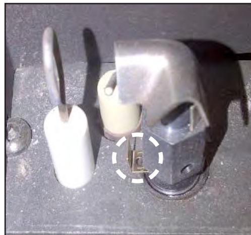
Figure 23. Pilot Slider set to LP
