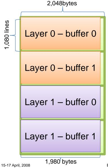
This is typical frame buffer allocation for 2 double buffered layers with CLUT8 in Full HD, i.e. 1980x1080x8bit.
