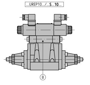
Directional spool valves type **UREP10...** may be provided with the pilot choke adjustment (8) as well as with accessories such as: spool stroke limiter (9) or or both optional accessories. Detailed information concerning depending on version of directional valve with accessories given on page 9-10.
