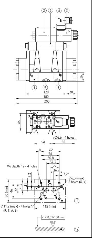
directional valve 12 - Subplate surface required
