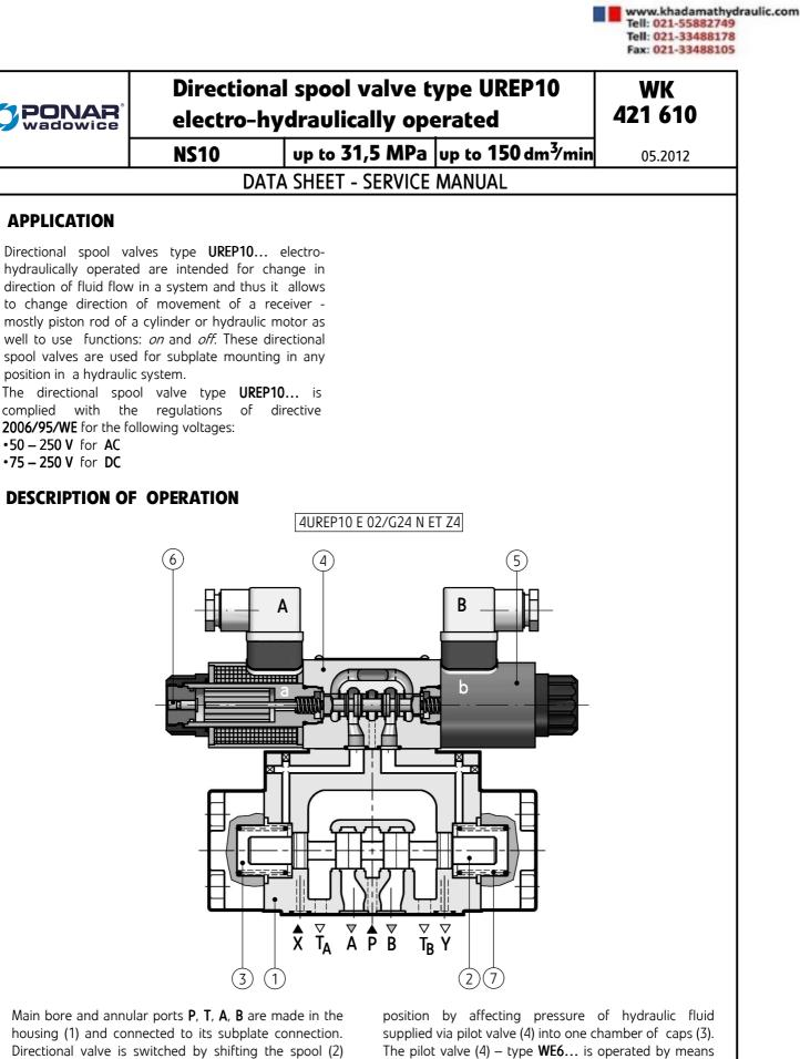
housing (1) and connected to its subplate connection. Directional valve is switched by shifting the spool (2) into one end position. Various control functions are dependent on the spool (2) which affects the change in configuration of connections among ports **P**, **T**, **A**, **B** in the housing (1). The spool (2) is shifted from its neutral
