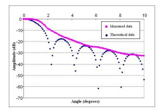
**Fig.8:** Theoretical and measured (experimental) directivity patterns on a logarithmic scale (dB scale) of the 3.5 MHz piezoelectric transducer
