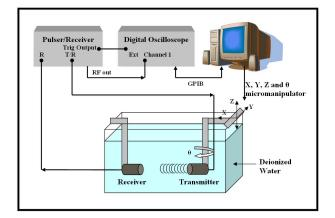
**Fig.1:** The experimental set-up for the directivity pattern measurement of ultrasonic transducers
