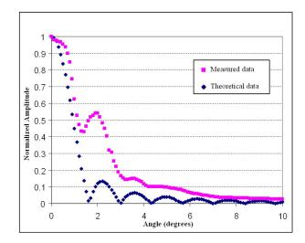
**Fig.6:** Theoretical and measured (experimental) directivity patterns on a linear scale of the 5 MHz piezoelectric transducer
