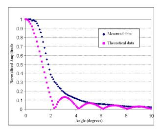
**Fig.5:** Theoretical and measured (experimental) directivity patterns on a linear scale of the 3.5 MHz piezoelectric transducer
