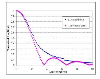
**Fig.4:** Theoretical and measured (experimental) directivity patterns on a linear scale of the 2.25 MHz piezoelectric transducer
