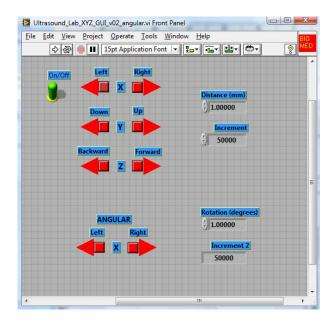
**Fig.2:** Custom-made LabVIEW program for the alignment  $(x, y, z \text{ and } \theta \text{ directions})$  of the transducers
