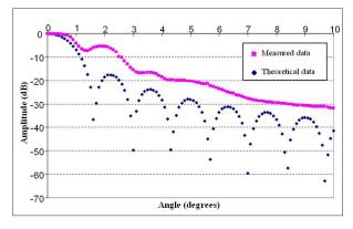
**Fig.9:** Theoretical and measured (experimental) directivity patterns on a logarithmic scale (dB scale) of the 5 MHz piezoelectric transducer
