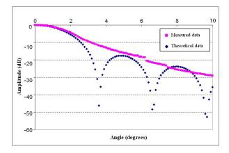
**Fig.7:** Theoretical and measured (experimental) directivity patterns on a logarithmic scale (dB scale) of the 2.25 MHz piezoelectric transducer
